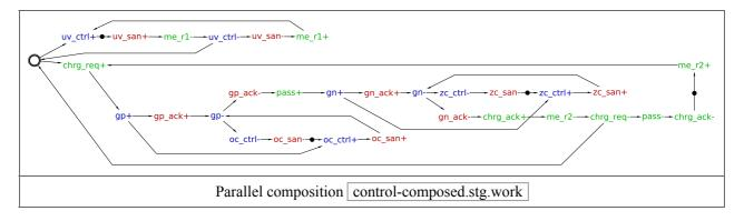
If you did not tick *Guaranteed N-way conformation* option, then the composed <u>STG</u> may have some redundant places (sometimes implicit within arcs). These places can be removed by resynthesis via *Conversion* $\rightarrow$ *Net synthesis [Petrify]* menu or individually, after checking their redundancy via *Check place redundancy* popup menu.
