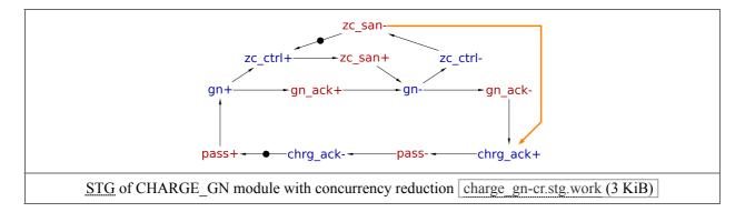
This concurrency reduction significantly simplifies the implementations of CHARGE\_GP and CHARGE\_GN, down to 60 units, so the area of the whole controller is reduced to 136 units. Using the composition technique the area can be further reduced down to 128 units (equivalent to removing a single inverter).
