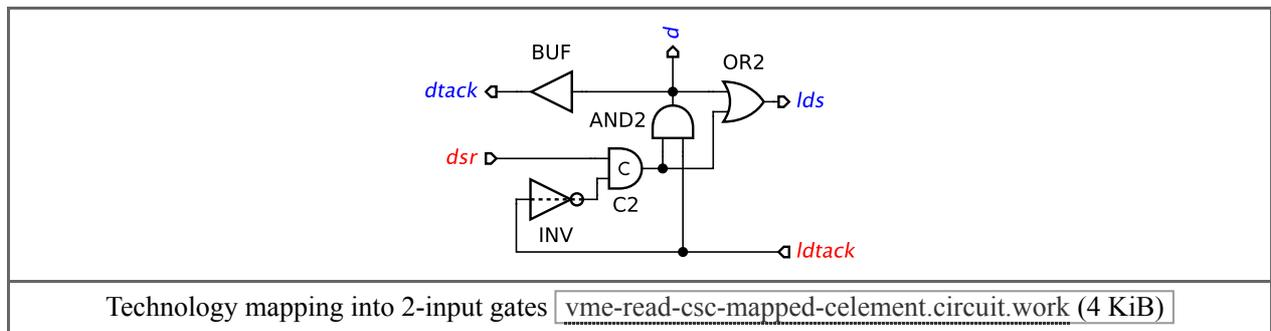
The circuit is now mapped – the gate labels correspond to the gate names in the library. Interestingly, MPSat replaced the 3-input gate with feedback by a latch. In fact, this replacement is not equivalent in the Boolean sense – there is a difference when  $dsr=ldtack=0$  and  $csc=1$ ; however, no such state is reachable, so this implementation is correct – this can (and should!) be formally verified using *Verification* menu.
