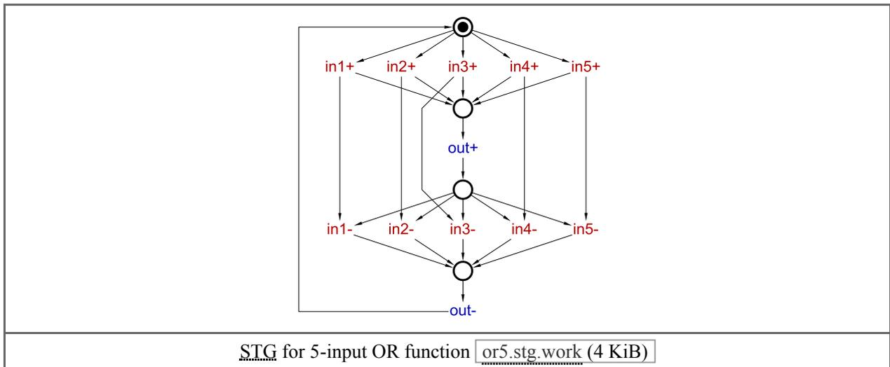
The complex-gate implementation is a 5-input OR gate as expected, but Workcraft's default gate library does not have an OR5 gate, and both Petriify and MPSat fail to decompose this example. If extending the gate library is an option, one can just add an OR5 gate to it. Unfortunately, expanding the library is rarely an option.
