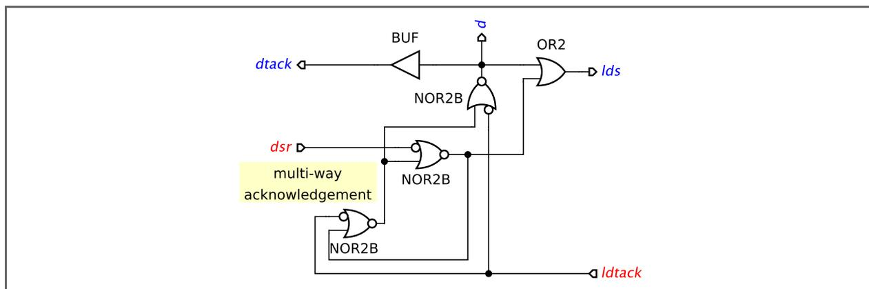
Technology mapping into 2-input combinational gates [vme-read-csc-mapped-2input.circuit.work \(4 KiB\)](#)
