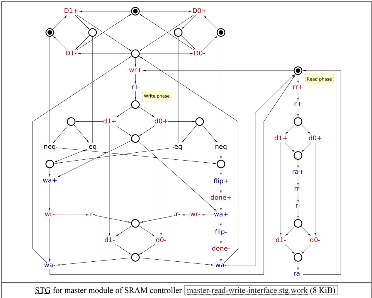
This STG has a rather contrived structure with many choice and merge places, and also has four dummy transitions (dummies are generally ‘difficult’ for some of the synthesis and verification tasks in Workcraft). Not surprisingly, MPSat fails to map this circuit; Petrifly at first seems to succeed, but the resulting circuit has gates with disconnected pins and fails the verification (looks like a bug in the tool).
