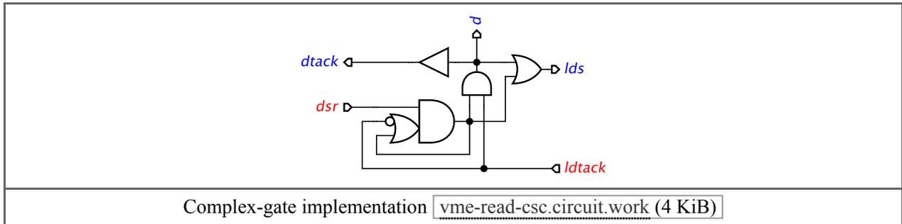
This circuit is not mapped yet, i.e. complex-gates are just Boolean functions of arbitrary size, e.g. they can be not implementable by any library gate. In this case, however, the STG was tiny and all the gates in the circuit are likely to be mappable to a realistic gate library.
