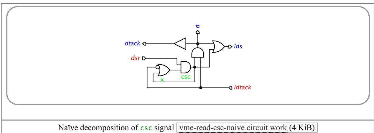
This can be done by right-clicking this gate and selecting *Split multi-level gate* from the pop-up menu. (Alternatively use *Transformation*→*Split multi-level gates (selected or all)* menu.) Unfortunately, the new delay associated with the output of bubble-OR gate breaks the speed-independence of the circuit, and it no longer satisfies the conformation and output persistency properties in the *Verification* menu.
