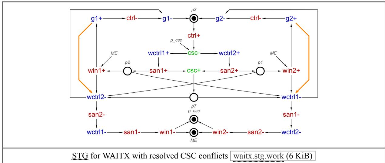
The following [STG](#) shows how to add two more concurrency reductions – the “high-level understanding of the design” allows one to conclude that these concurrency reductions are unlikely to harm the performance. The modified [STG](#) turns out to be much easier to map and the circuit is better (the area is 156 units for MPSat and 152 for Petrify – you may get different results) with much smaller gates (the circuit in [3] was then slightly improved manually).
