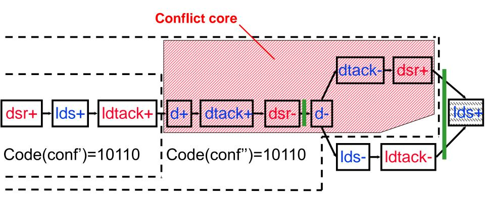
Idea: Insert csc+ into the core and csc- outside the core to break the balance
