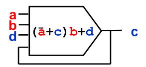
Signals that are the inputs of the gate producing a signal form its **support**, e.g. the support of c is {a,b,c,d}. Supports are not unique in general.
