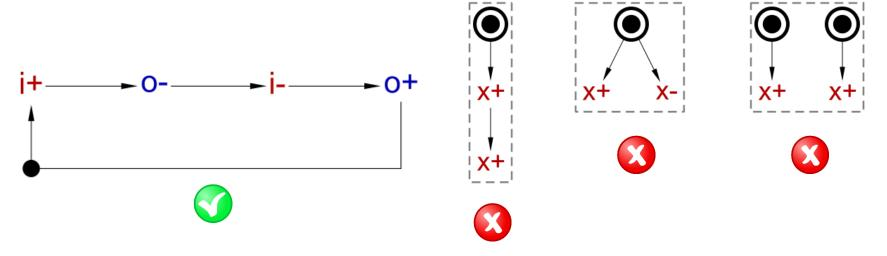
Output-persistency: an enabled output must not be disabled by another signal firing first
